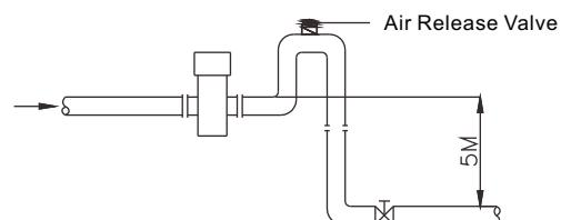
6. The control valve and cut valve should be installed at the downstream of the sensor rather than the upstream.
