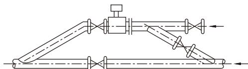
14. When installing the sensor, it should ensure that the measuring pipe and the process pipe must be on the same axial line. For the flow meter with the pipe meter of 50mm or below, the axial line deviation should not exceed 2mm. For those of DN65~DN150, the axial line deviation should not exceed 3mm. For those of ≥DN200, the axial line deviation should not exceed 4mm.
