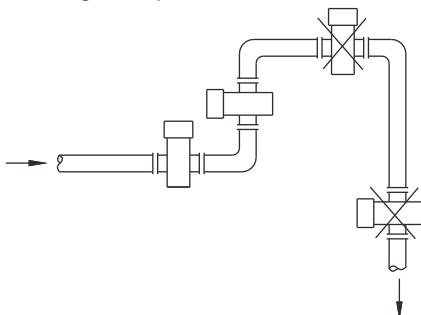
3. It should be installed at the rising point of the pipe.
